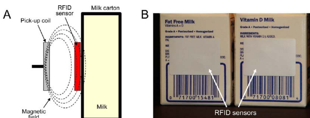
Figure 4. RFID sensor layout for demonstration of determination of milk freshness: (A) schematic of sensor positioning onto a milk carton and sensor-response readout with a pick-up coil; (B) photograph of milk cartons with attached RFID sensors.
